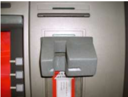
2. Close up of card reader attachment over card slot
