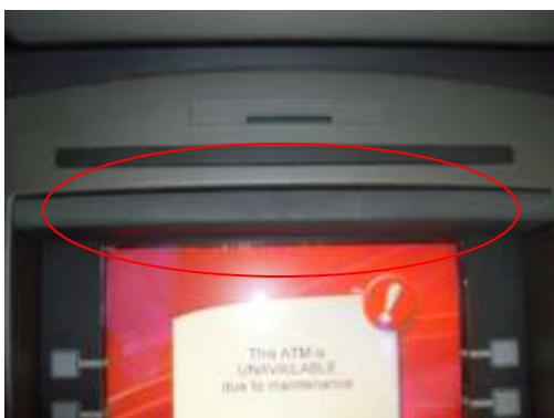
3. Close up of pinhole camera housing
